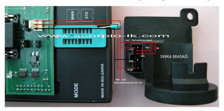
The device provides advanced features as well as basic mode. The basic mode intended for keys producing and described below. The advanced mode is for engineer purposes and isn't described in this document.
