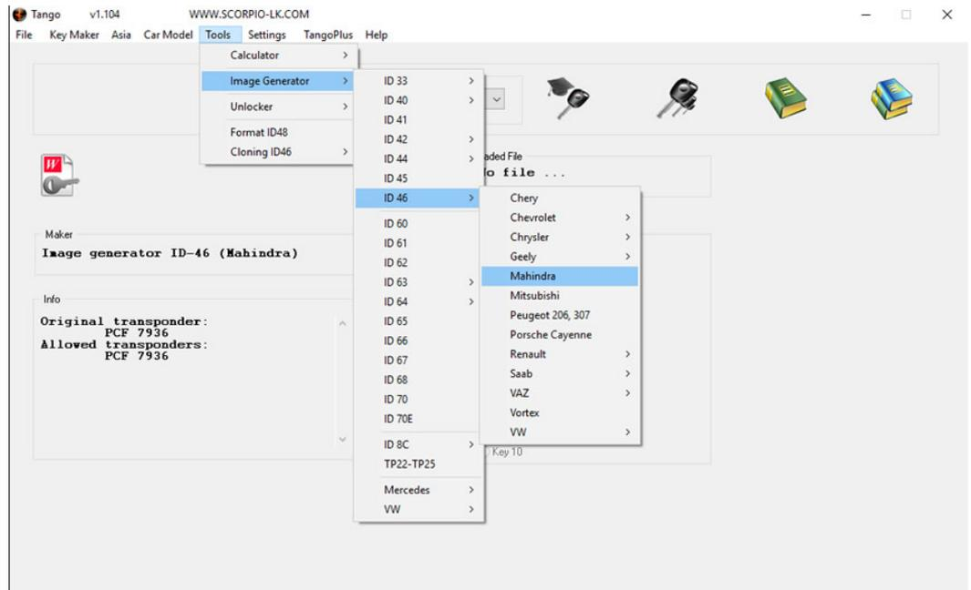
After that place transponder in coil and select appropriate key type - XYLO or Scorpio depending on the immobilizer you are working on
