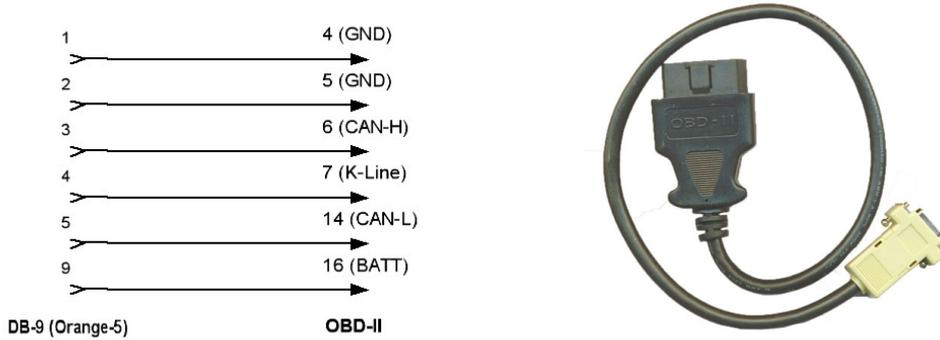
Work can be performed directly with the immobilizer drawn-out of the car using the following wiring diagram:
