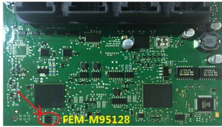
Picture 1: EEPROM position on FEM System
