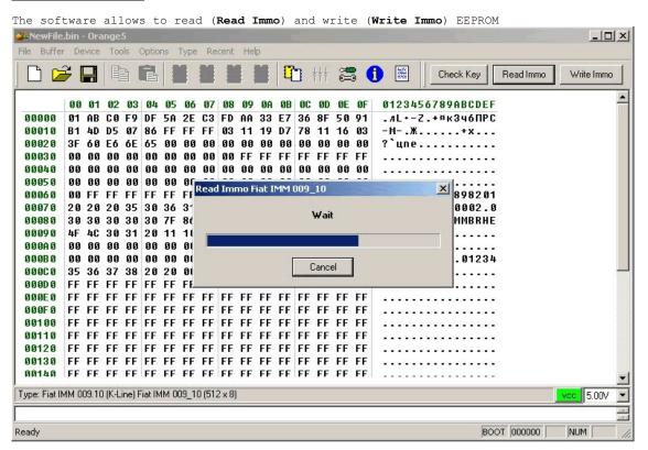
After successful read and save of the dump data file a new transponder can be created through the function built in Tango programmer. After that write back to the immobilizer the file generated by Tango programmer.
